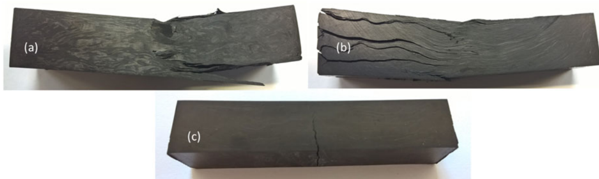
Figure 12. The various failure mechanisms observed in the Short Beam Shear tests, showing (a) tensile failure in an edge sample, (b) shear failure in a central sample, and (c) matrix failure in a knit line sample.
