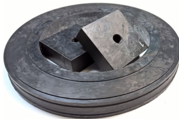
Figure 1. A demonstration of the machinability of MC1200/AS4 DFMC, showing a series of lathe-made cuts on a ring and two 5/16 th threaded holes tapped into plates.
