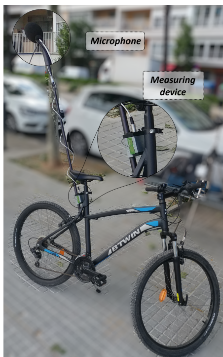
FIG. 5.6: Bike with the GNS mounted in the lower part of the seat. The microphone is located at the top of a tube at an approximated height of 2 m.
