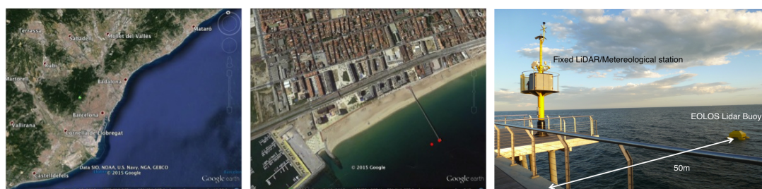
Figure 1.6: PdP test campaign site. (a) Location of the test site near Barcelona coast (Badalona). Red dots denote the position where the “fixed” and “floating” lidars have been placed. (b) Plan view PdP test site. (c) Meteorological tower and EOLOS Doppler lidar buoy.
