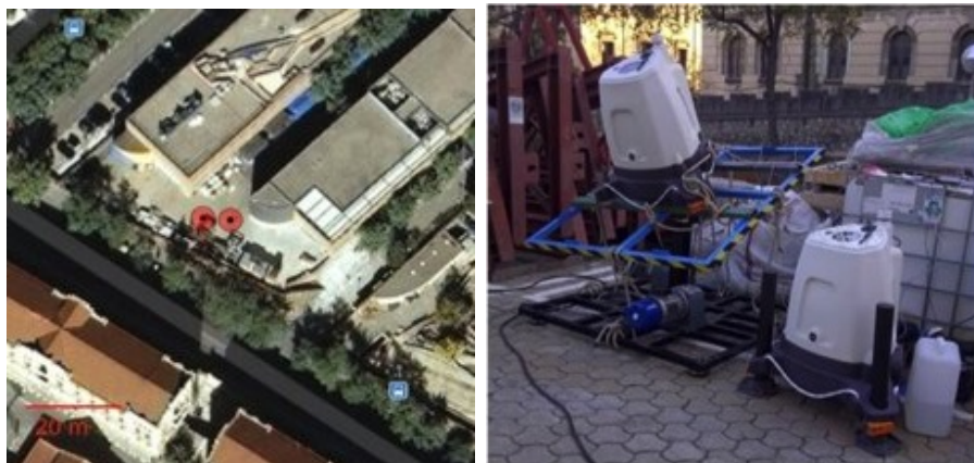
Figure 1.5: LIM - UPC test campaign. (a) Plan view of experimental set up at LIM/UPC premises (b) Experimental set up showing the reference “fixed” lidar and the moving “floating” lidar on the motion simulator platform.
