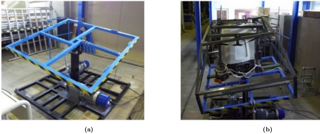
Figure 3.3: Motion simulator and experimental test setup. (a) Motion platform used to simulated pitch and roll tilting. (b) Cardan frame used to counter-balance the motion applied by the platform simulator. Both the motion-simulation platform and the cardan frame have been developed by the Maritime Engineering Lab (LIM-UPC).
