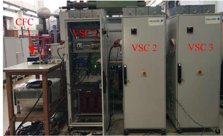
Fig. 5.22: Image of the experimental platform, including the CFC and the three VSCs.
