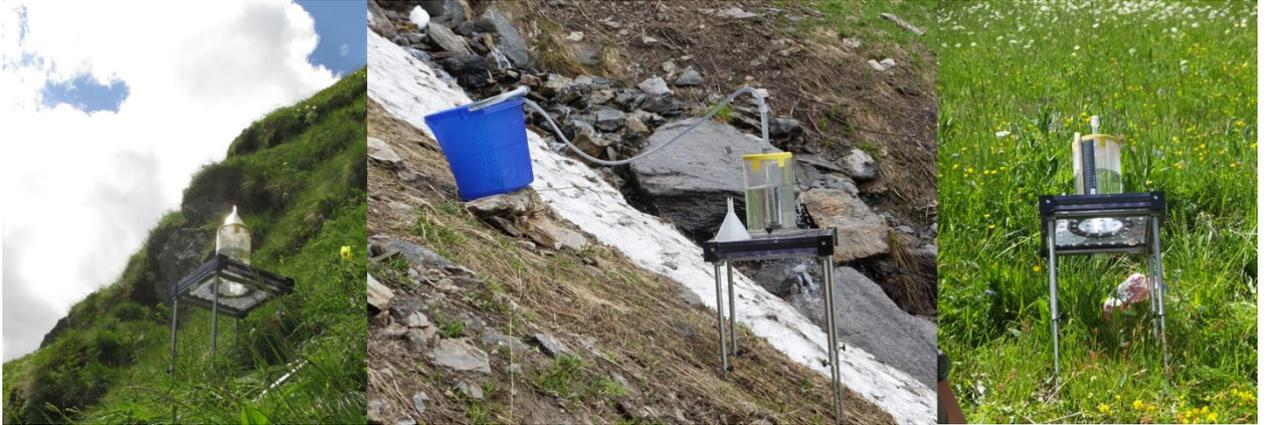
Fig. 6.1: Different setups and preconditions of the rainfall simulation experiment on steep slopes in Val Piora, Ticino, Switzerland
