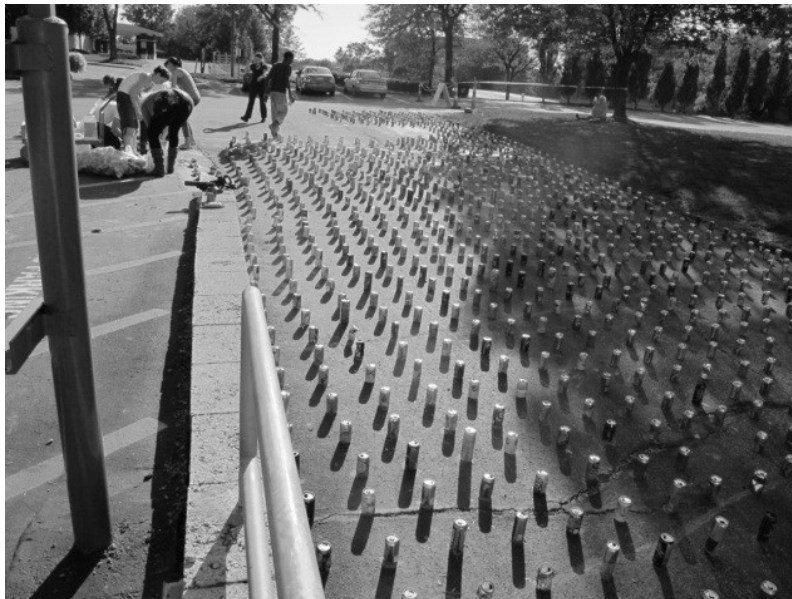
Figure 2. Recycled 12 ounce cans were filled with water and placed on top of the 1' grid of blue dots. Twelve ounces per square foot represent approximately 1/6" of rain.
