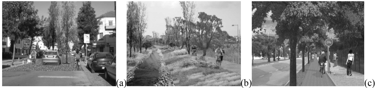
Figure 28 - Scene of proposed traffic calming designing measures for Almada Cycle Network coexistence between bicycles (a); pedestrians typology along qualified greenway in Almada Cycle Network (Magalhães & Mata, 2005b) (b) and typology - separated bicycles from pedestrians – in implemented cycleway plan for Almada Cycle Network (c) (Magalhães et al , 2005a)
