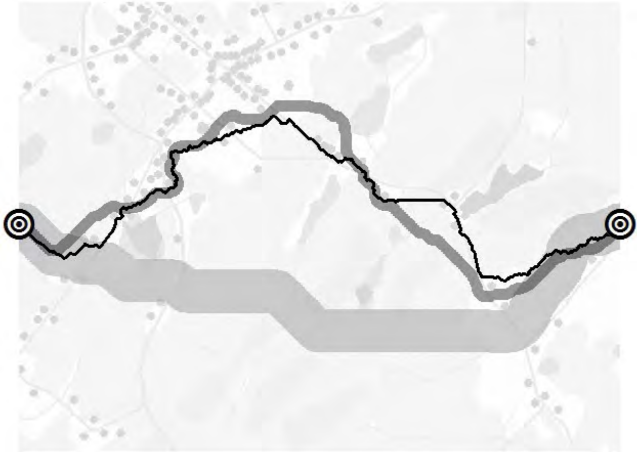
Fig. 3. Minimum-cost Corridors of Different Widths. The relative cost of traversing each location within a geographical area is indicated in pale gray, with darker shades corresponding to higher costs. The linear corridor in black connects the two termini depicted as concentric black circles with the lowest possible sum of those incremental costs. The wider corridor in dark gray and the even-wider corridor in a lighter shade of dark gray do the same, given that each of the corridors must maintain a specified width.
