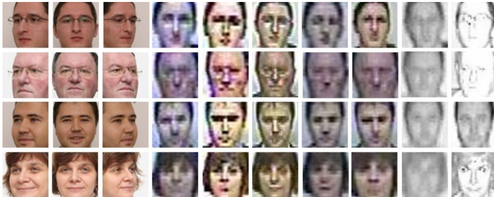
Figure 3: Faces detected by the Viola and Jones face detection algorithm of four individuals from the challenging SCFace Dataset (Grgic et al., 2011). The first three columns show the Gallery images while the remaining columns show the test images. The large difference between the quality of the gallery and test images is evident.
