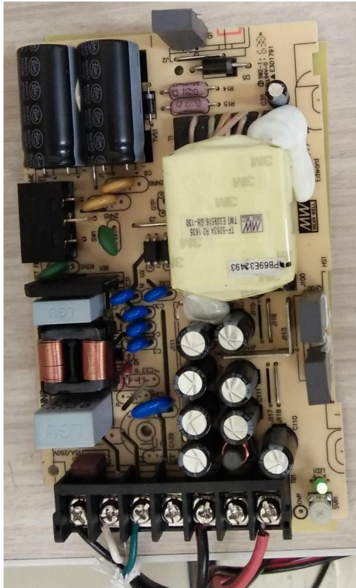
Figure 5-4 12V DC power supply to power-up the radio-set and protecting against surges
