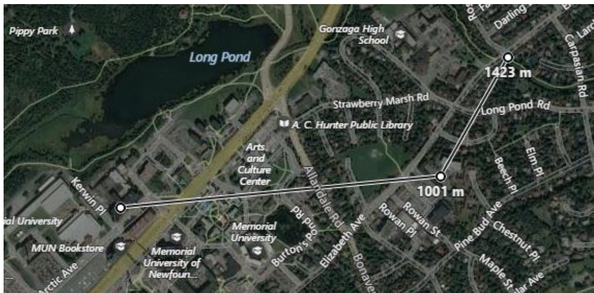
Figure 4-15 Range testing in obstacle dense area after implementing a mesh network
