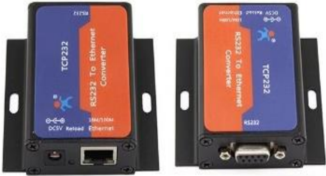
Figure 5-6 USR-TCP-232 used in the project for serial to ethernet conversion
