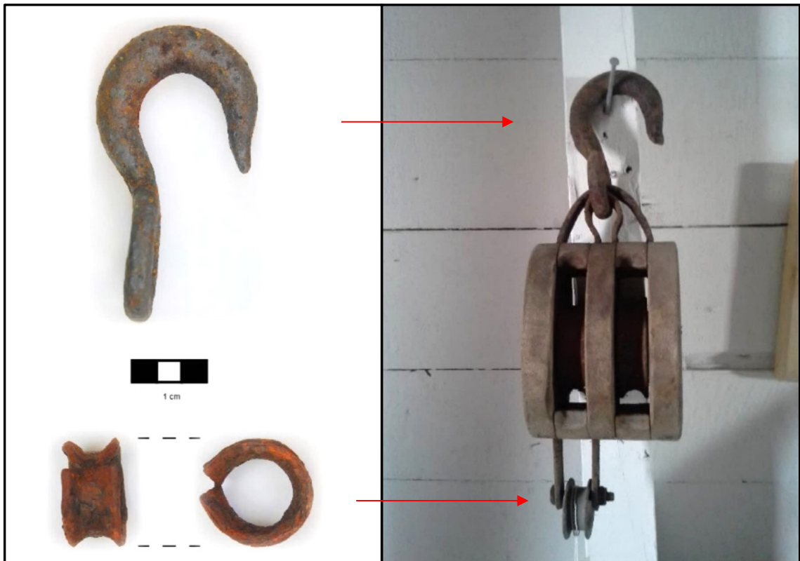
Figure 6.7 Iron hook and one iron thimble beside example of block and tackle at Netloft Museum, Rigolet.
