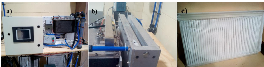
Figs. 3. a) Lab-scale AGMD system; b) solid steel casing; and c) membrane cassette to be placed in the solid steel casing.
