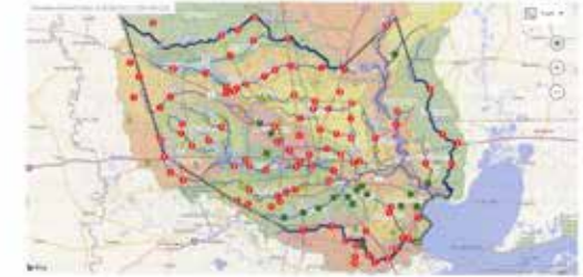
Figure 4.5. Status of the HGFC stream gages as of August 28, 2017 12:00 AM (CDT). Locations marked in red are out of bank and locations in yellow are near the top of bank. Figure courtesy of Mps (www.harriscountytexas.org).
