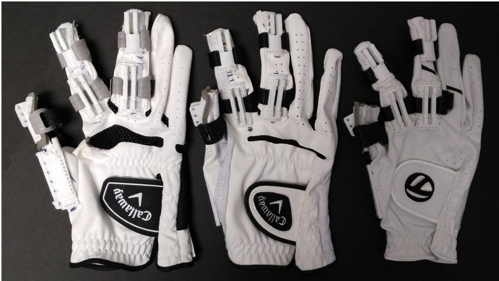
Figure 6.1: We developed a customized glove to interface hands with a rigid link mechanism of exoskeleton. Depending on the size of a subject's hand, one among three different sizes of gloves is selected.
