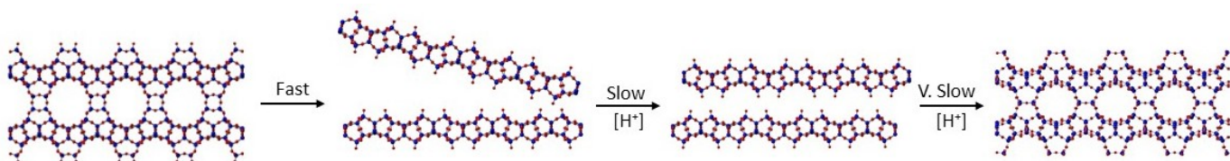
Fig. 1. A schematic representation of the ADOR process from parent germanosilicate UTL . Step 1 proceeds through the fast hydrolysis in water to form the disordered IPC-1P layers. Upon treatment with hydrochloric acid these layers begin to rearrange themselves (step 2). Finally, in step 3, the rearrangement is coming to an end and the new daughter zeolite is beginning to be formed. Upon calcination IPC-2 (shown here) would be afforded. The rate of the final two steps are greatly increased by an increase in molarity of acid, [H^+] .
