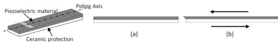
Figure 4.13: Schematics of the shear transducer. (a) Undeformed, (b) Deformed.
