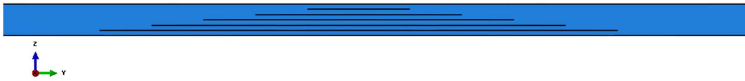
Figure 7.3: Cross section of the plate to show the pyramid-like impact damage geometry. Top side is the impact surface. Delamination size increases as we move to the bottom surface.
