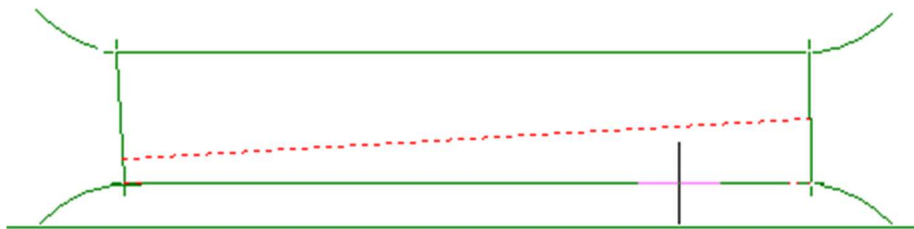
Figure 17. Geometry Calculated by the Micro-Vu Machine. Note that the gauge length, shown by the dashed line, must be calculated indirectly.
