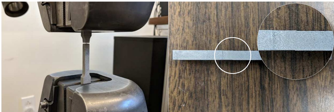
Figure 24. Printing Error in Location Influence Samples. Left: A failed specimen after tensile testing. Right: The root cause of the failure was a subtle offset between the geometries printed before and after the machine paused.
