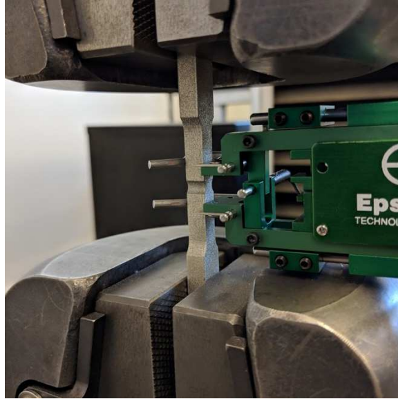
Figure 26. Experimental Setup for Notched Specimens. Similar to the baseline, an extensometer was used to measure elastic displacement.
