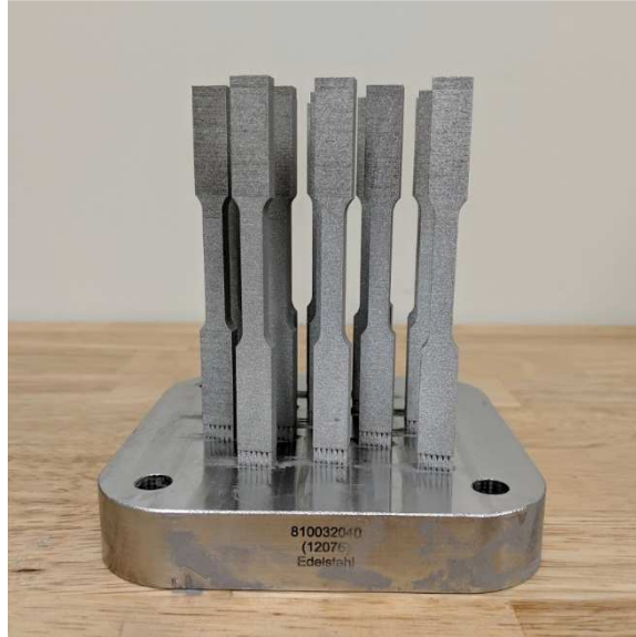
Figure 9. As-Printed Tensile Specimens. Printing in the Z-direction minimizes the amount of support material required.
