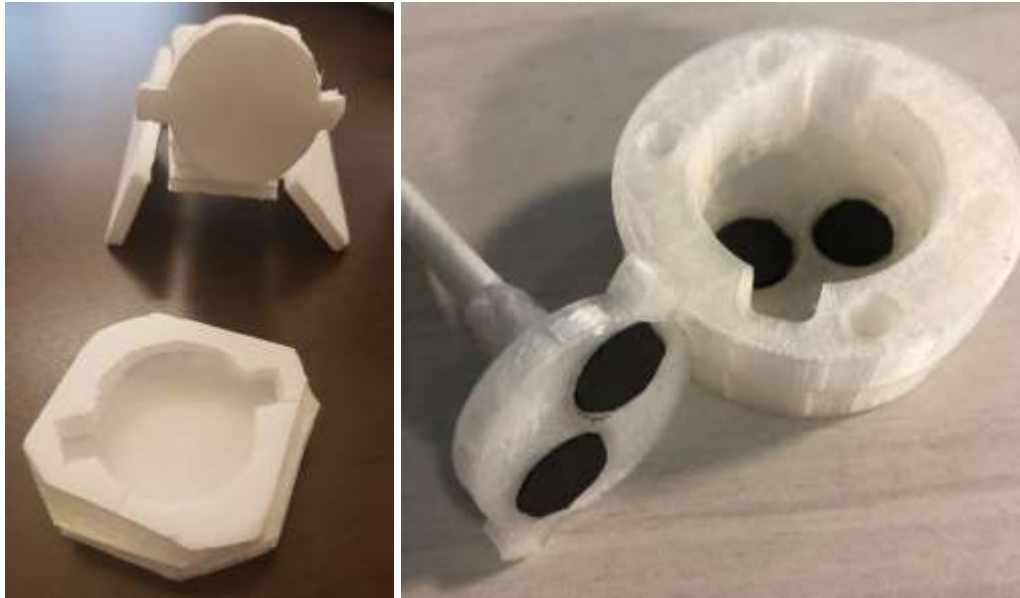
Figure 6.2) Initial models of the quick-change wrist; (left) foam core model; (right) 3D printed model with embedded magnets
