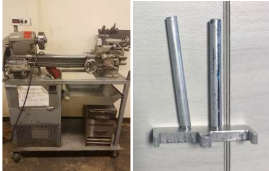
Figure 8.2) Manual lathe manufacturing (left) mini-lathe located in Mustang 60 (right) results of when threads misaligned versus aligned properly
