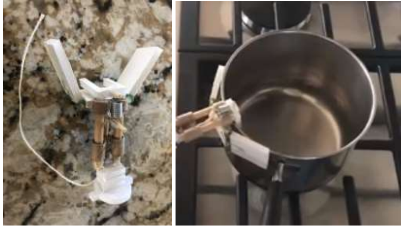
Figure 6.4) Foam core model of the body-powered clamp; (left) picture of clamp model; (right) clamp on lip of pot
