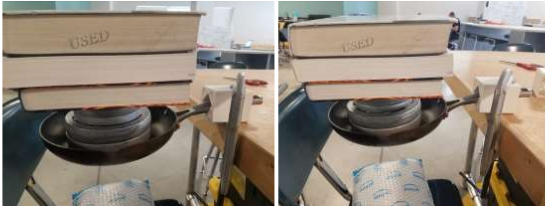
Figure 7.7) Preliminary sleeve testing with 75% infill density (left) and 50% infill density (right)
