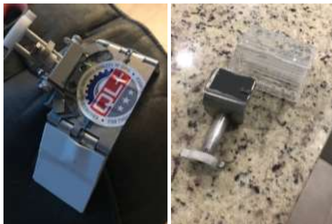
Figure 9.7) Broken prototypes: clamp arrived broken (left), cutting tool bracket came off during use (right)
