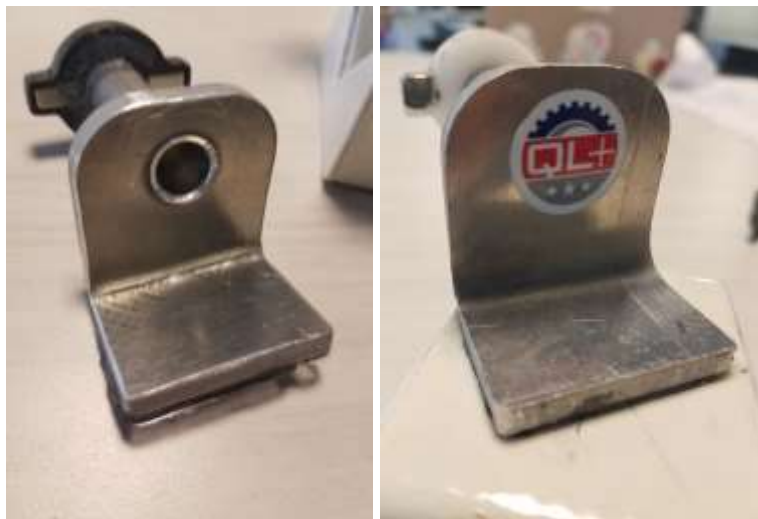
Figure 8.5) Cracked aluminum 6061-T6 sleeve bracket (left) and final aluminum 5052-H32 sleeve bracket (right)
