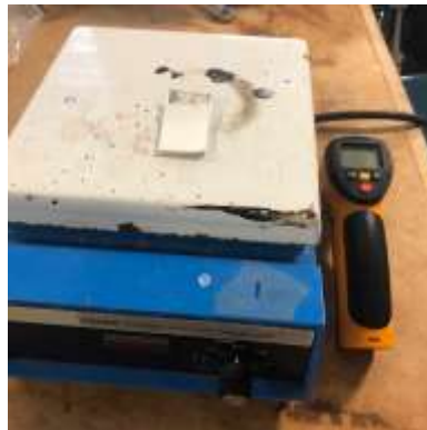
Figure 9.3) Silicone coating thermal characterization test setup
