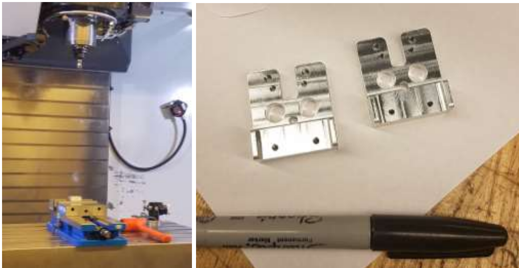
Figure 8.3) Central attachment point manufacturing; (left) CNC setup ready to start machining; (right) finished central attachment points with sharpie for size reference
