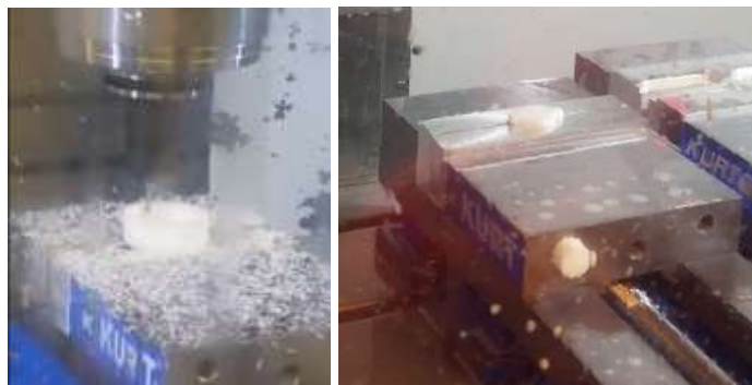
Figure 8.1) CNC machined wrist base process
