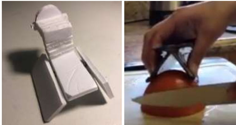
Figure 6.8) Initial cutting tool prototypes; (left) foam core cutting tool model, (right) updated triangular model testing
