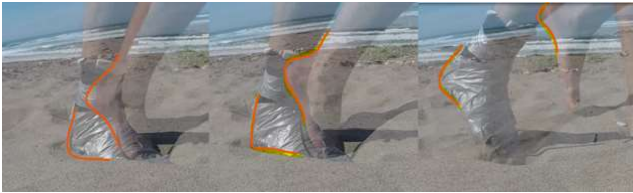
(a) (b) (c) Figure 4: Walking on dry sand with and without a flexing ankle and toes
