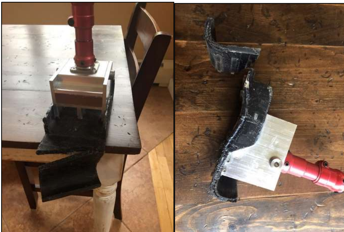
Figure 10: Carbon Fiber Sole Longitudinal Crack
