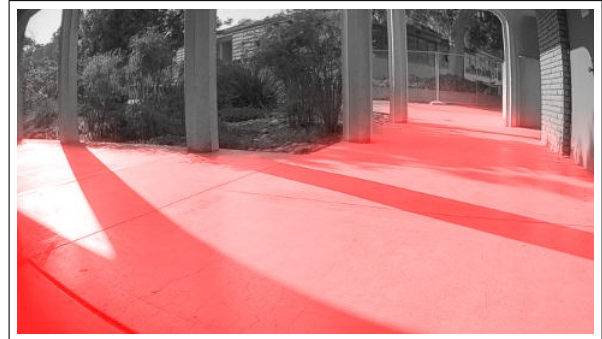
Fig. 3. A generated path mask for a given input image passed to the neural network with output space 480x270
