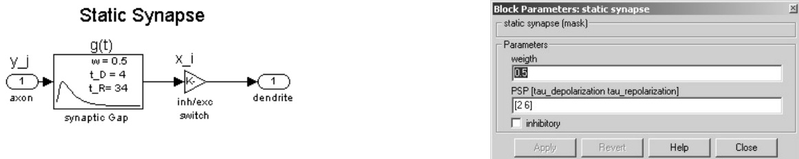
Figure 3.3: left Panel - structural layer of the neural base library element static synapse right Panel - parametric layer of the static synapse base element.
