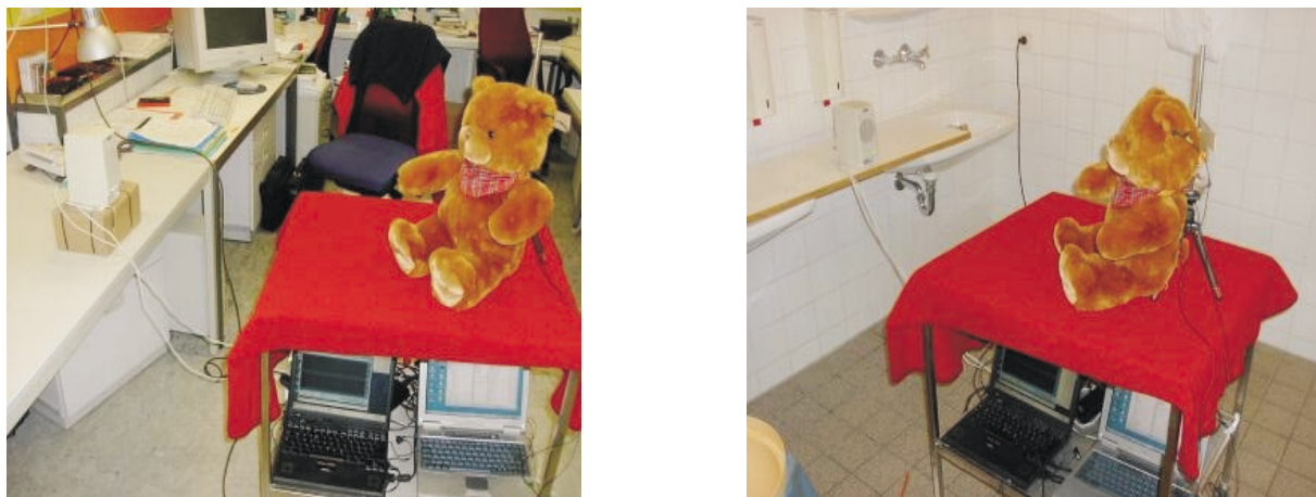
Figure 5.28: Experimental setup for the recording of real world signals, using a Teddy with an ear base of 20 cm and two microphones in front of a single speaker at about 1.5 m distance.
