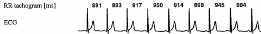
Figure 10: Example of an RR tachogram derived from the ECG raw data. Intervals between two R-waves are displayed in ms.
