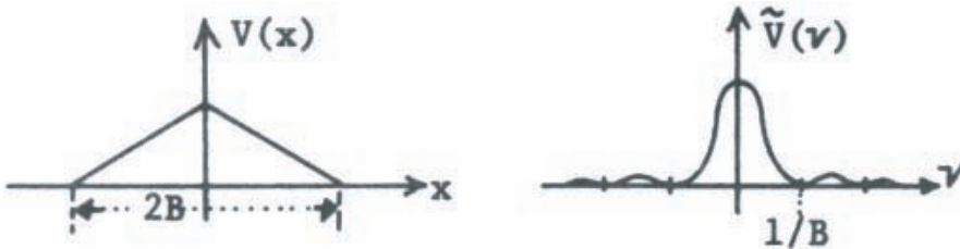
Figure 15.2: The trian-function and its Fourier transform.
