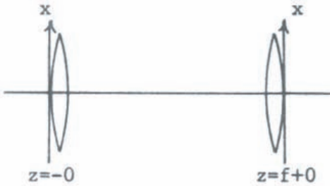
Figure 22.5: The configuration of the “light tube” for generating Fraunhofer diffraction.
