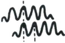
Figure 33.5: Interference of two wavefronts shifted by one wavelength.
