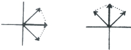
Figure 31.8: Vector decomposition of the incident polarization directions.
