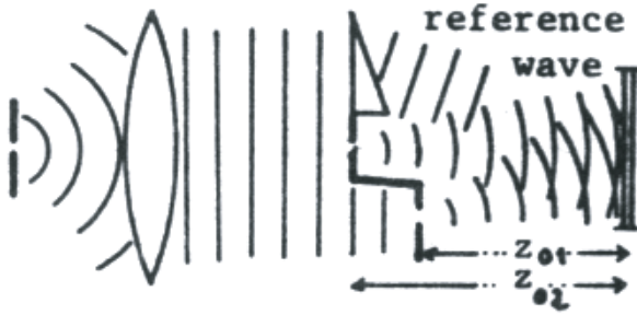
Figure 32.21: Object with two points at different depth positions.
