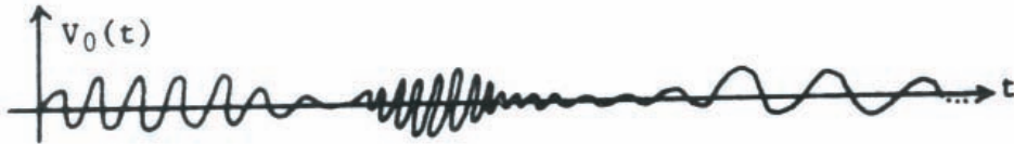
Figure 33.11: Short pulses as a model for white light.
