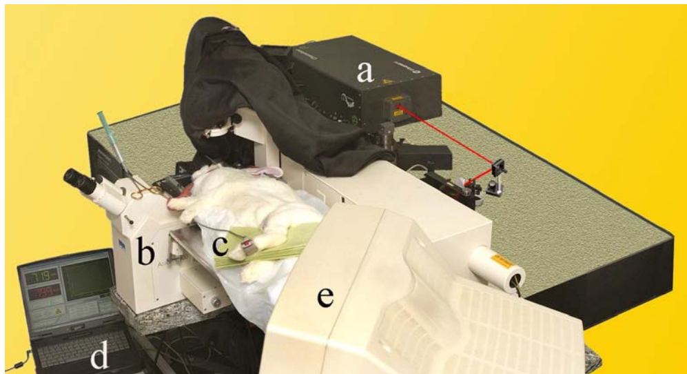
Fig.12_1 Modified photograph of operations on rabbit depicting the integrated system involving the laser head Chameleon and the modified Zeiss multiphoton microscope. The optical mirrors deflecting the laser beam are here illustrated with a simple way. a: Compact tunable non-amplified 90MHz Ti:sapphire Chameleon; b: Multiphoton microscope based on inverted Zeiss LSM 410; c: The animal on animal bed in operation; d: Wavelength tuner; e: Imaging-monitor.
