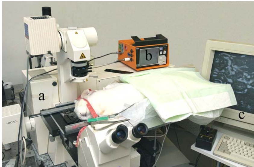
Fig.12 Photographic illustration of laser eye surgery with rabbit based on a modified Zeiss inverted laser scanning microscope integrated with a compact non-amplified 80 MHz Ti: sapphire femtosecond laser. a: Multiphoton-microscope; b: Draeger dialogue 2000; c: Imaging monitor.
