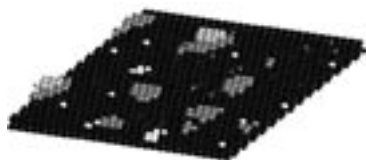
Fig. 2: Simulated Si-(111) surface after deposition of 12% of a C monolayer. Black and white spheres denote substrate atoms and vacancies created by thermal fluctuations, respectively. Dark grey spheres denote C atoms incorporated into the substrate. Atoms that are combined into the clusters are shown in light grey (lighter tint is used for upper cluster layers).
