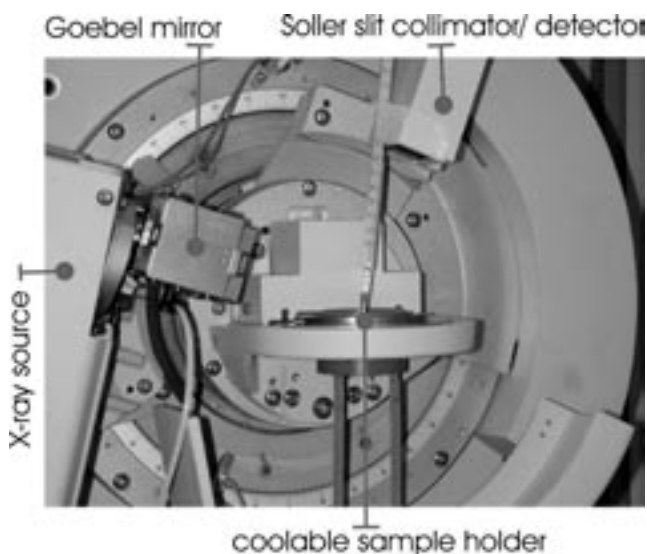
Fig. 1: Theta-theta diffractometer equipped with special sample holder operated by liquid circulation cooling (detector not in measuring position)
