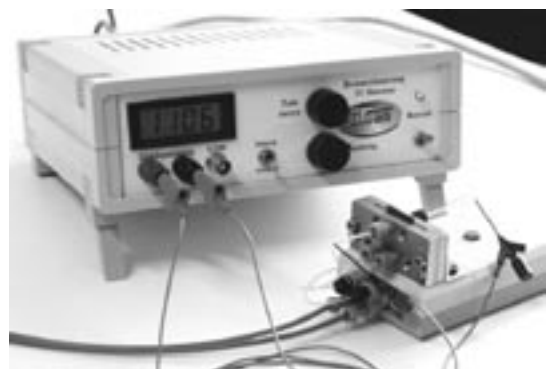
Fig. 3: Actual setup of microcombustor with control unit, electrodes and gas supply
