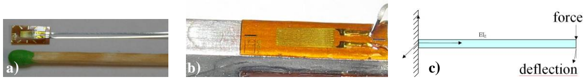
Fig. 1: a) Strain gauge 1-LY11-3/350, b) Measuring area of the strain gauge c) Test setup
