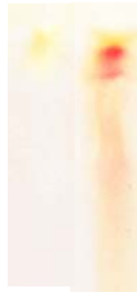
Fig. 4: Nickel sequestering compounds exuded into the medium. Thin layer chromatography of medium after growth of nickel resistant strain S. acidiscabies E13 from Wismut soil in media lacking (left) and containing 1 mM nickel (right). The chromatogram was stained with nickel specific dimethylglyoxime giving a red stain. The uppermost, brown-colored band is assumed to be melanin.
