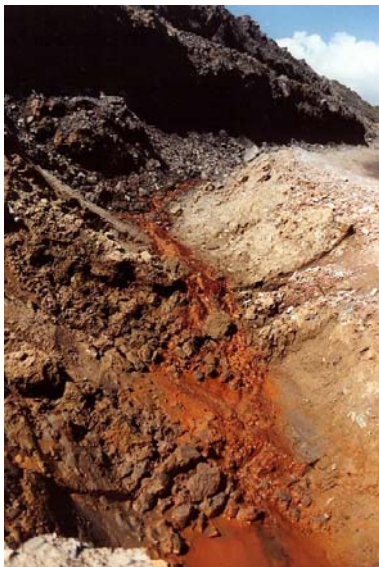
Figure 1: AMD formation at a former uranium mining site in Thuringia. Photo: S. Senitz.
