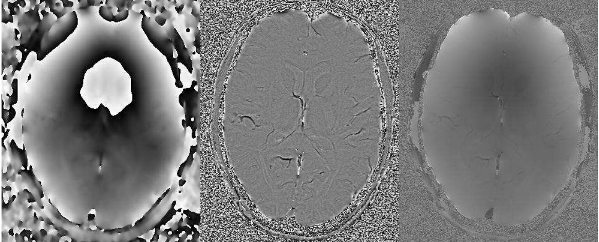
Figure 3.2: Left: Phase of the low pass filtered complex image from Fig. 3.1. Middle: Homodyne filtered phase image obtained by complex division of the original and low pass filtered image. Right: Unwrapped phase image obtained by a region growing algorithm.
