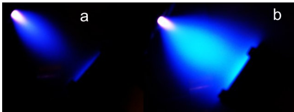
Figure 4.21: Photos of plasma plume from ZnO: a) 1 Pa oxygen pressure b) 10 Pa oxygen pressure.
