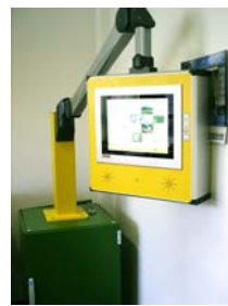
Figure 6: Barrier-free stationary info-terminals with a possibility of direct query at the terminal (see left fig.), the feasibility to connect with several back-ends over WLAN, Bluetooth or infrared
