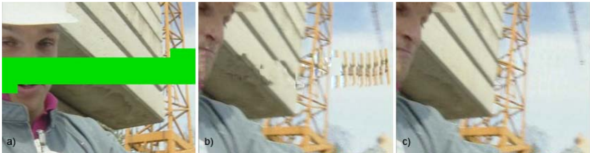
Figure 5 Lost macro blocks (a), error propagation (b) and resulting picture with I-block insertion (c)
