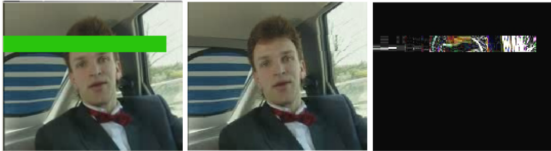
Figure 10 Lost macro-blocks (left), interpolated picture (middle) and amplified difference decoded original vs. interpolated picture (right)
