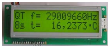
Figure 19. System local conversion (QT sensor) LCD display captures.
