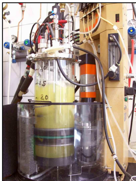
Figure 16. Fermentation of P. putida mt-2 using the reactor Labfors (Infors AG) using toluene as carbon source.
