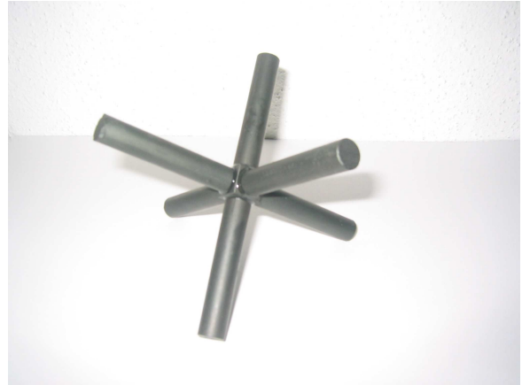
Figure 7 Ferrite core of the 3 D antenna. The length of the three rods is approximately 110 mm.
