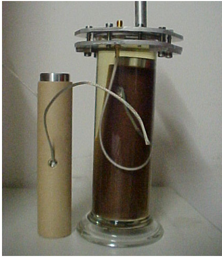
Figure 6: Prototype of a bushing model for the ageing investigations under different conditions.
