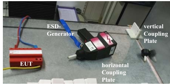
Figure 7 – Test Setup for ESD-tests
