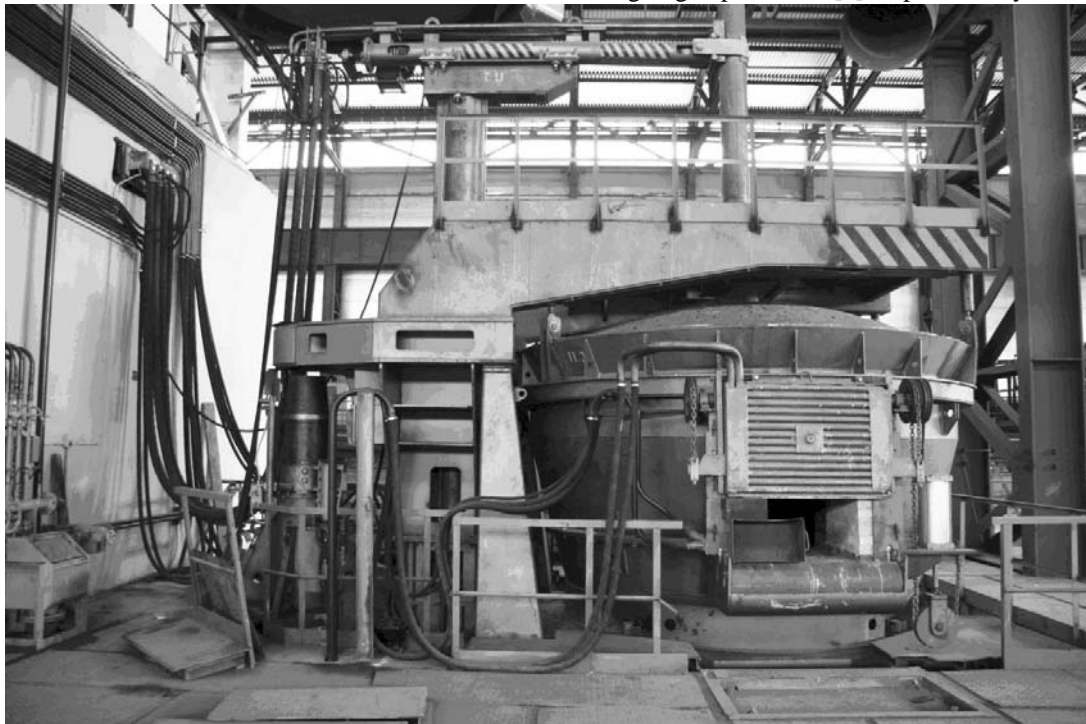
Figure 1 Direct Current Arc Furnace DPS-12
