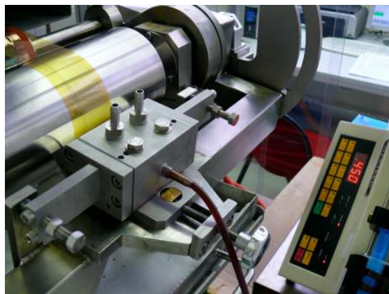
Figure 1: Slot die coating of low viscosity solution P3HT:PCBM (xylene, 1 m/min, 5 cm on PET/ITO foil with 2 m/min R2R coated PEDOT:PSS) at TITK e.V. coating machine LBA-200 (left) and I/V-characteristics of flexible solar cells; system: PET/ITO/ PEDOT:PSS- R2R (2 m/min) /P3HT:PCBM- R2R (1 m/min; different solvents) /Al; AM1.5, cell size 0.25 cm 2 (right)
