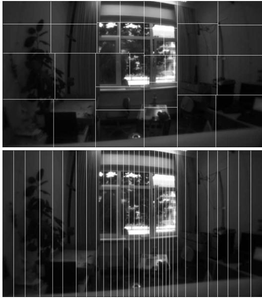
Fig. 2. Median cut algorithm for sufficiently exposed images. The subsections are distributed more evenly over the image.
