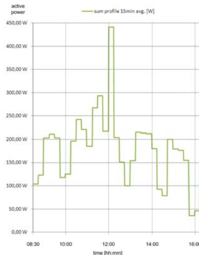
Fig. 4. Sum load profil of active power consumption of various appliances measured by a smart meter (15-minute mean values).
