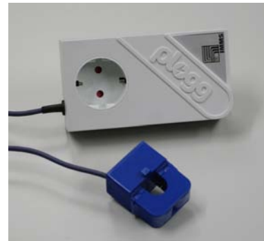
Fig. 2. BAsE-Meter with an external current clamp.
