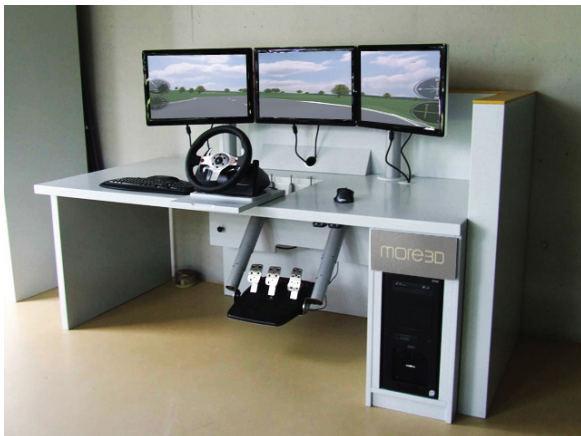
Figure 17 Prototype of a new design workplace in the scenario of driving simulation
