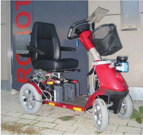
Fig. 3. The current mobility scooter equipped with electronics and sensors
