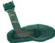
Figure 7. A foot sensors insole
