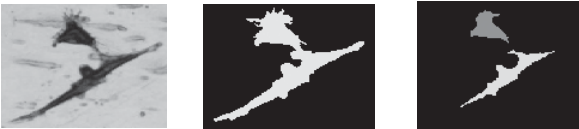
Figure 3: Erosion of a blob. After two iterations the blob separation will occur indicating that it must be a cell cluster
