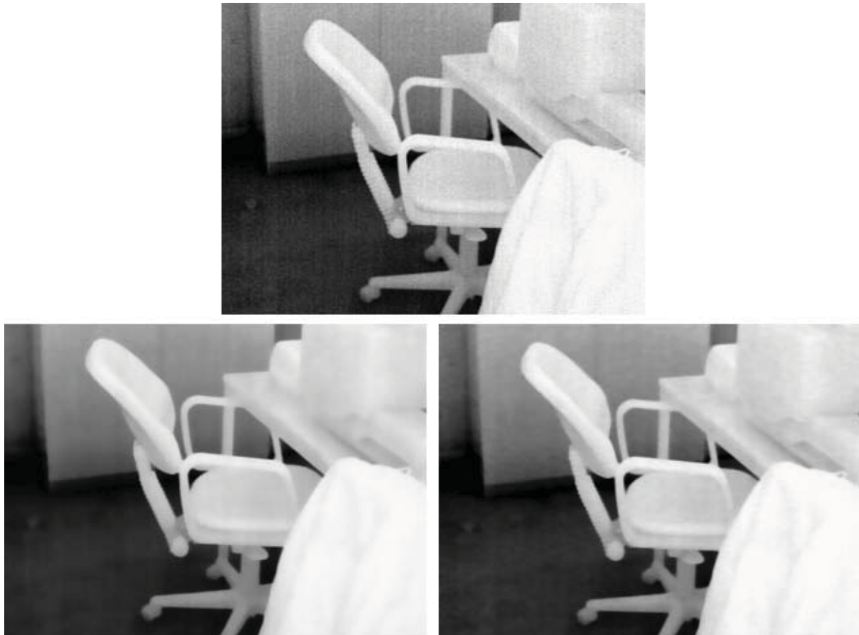
Fig. 3. Anisotropic Diffusion (AD) and Geometrical Filter (GF) , Original Image(above), Corrected image AD with 10 iterations(bottom left), Corrected image GF with 4 iterations(bottom right)
