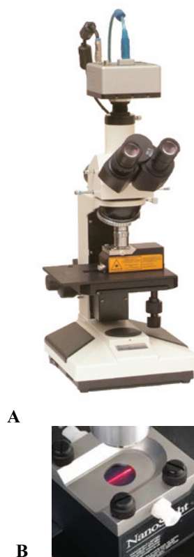
Fig. 1. The NanoSight™ device. A: microscopic arrangement; B: laser beam observed by microscope.
