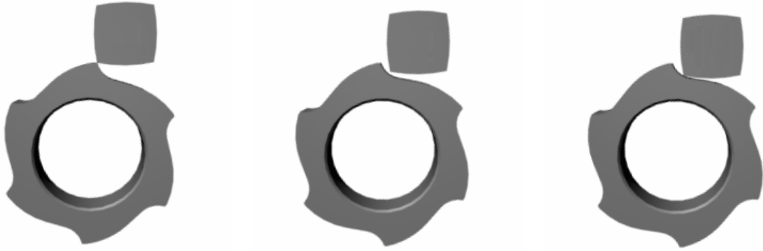
Figure 4 - Illustration of the contact loss between the follower and the cam.
