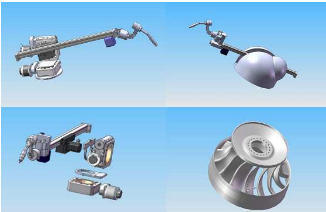
Fig. 2 – Robot prototype assembled and compared with the turbine model.
