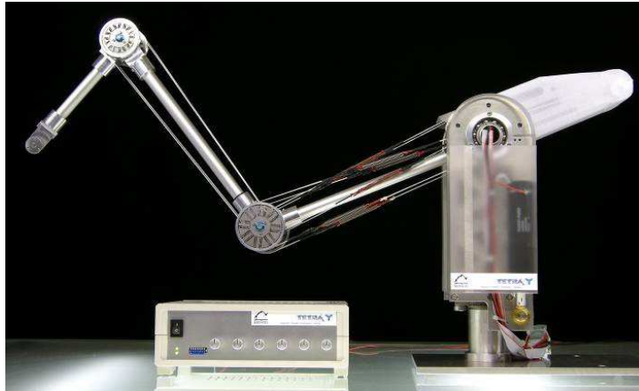
Figure 2: Design of the new BioRob arm with 4 DOF
