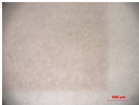
Fig. 3: Gravure printed structures using a photo structured glass cliché, ITO on a PET substrate (left), P3HT on a PET substrate (right)
